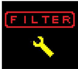
After 600 compressor running hours the filter must be cleaned.
