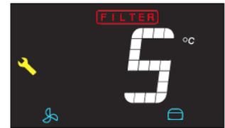
After 675 compressor running hours the alarm symbol
