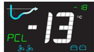
When the desired value is attained, an acoustic signal will be emitted. After the signal, defrosting is commenced (if such is required based upon the evaporator sensor's temperature). Then it subsequently switches to the storage program. Hence the desired value for the storage program must always be set and checked before starting "PCL"!
