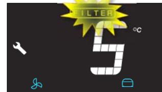
After 650 compressor running hours "FILTER" flashes red and the service symbol lights
