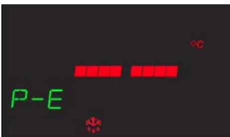
**Sensor defective or not connected**
