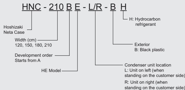
Powered by R600a Natural Refrigerant, energy efficient and sustainable, with a GWP = 3. Energy savings may vary depending on electrical specs when compared to HFC equivalent model.
