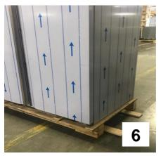
4-5-6) The other side of the long wooden pieces is moved to the right side of the refrigerator and detached from the bottom of the pallet with the help of a screwdriver.
