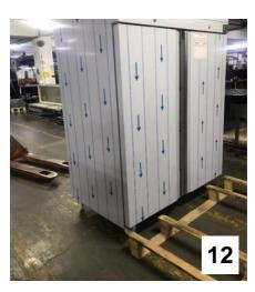
10-11-12) With the help of a pallet truck or by means of 2 people, the cabinet is first tilted to one side from the pallet and then the pallet is removed from the bottom. After the pallet leaves the refrigerator, the refrigerator is left slowly and with its feet evenly on the floor.
