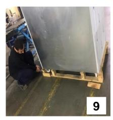
7-8-9) Then, 2 pieces of short wooden pieces at the back of the pallet are removed by hand. Once the pieces of wood that hold the cabinet to the pallet are removed, it means the cabinet is no longer connected to the pallet.
